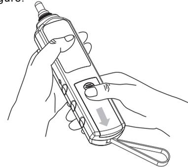
b. Insert the 9V battery into battery compartment, note the battery polarity, and then close the battery door, as shown in following figure:
