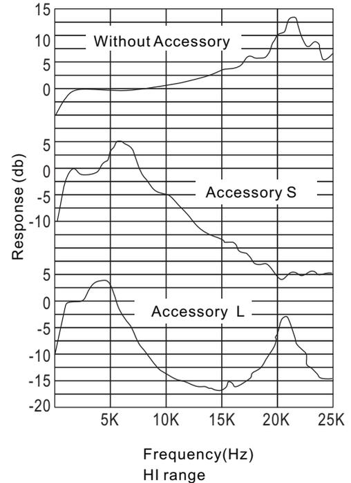
8. Contact resonance in acceleration measurement:
